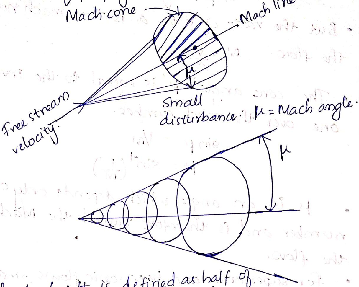
④ **Mach Angle:** It is defined as half of propagation speed of sound.
