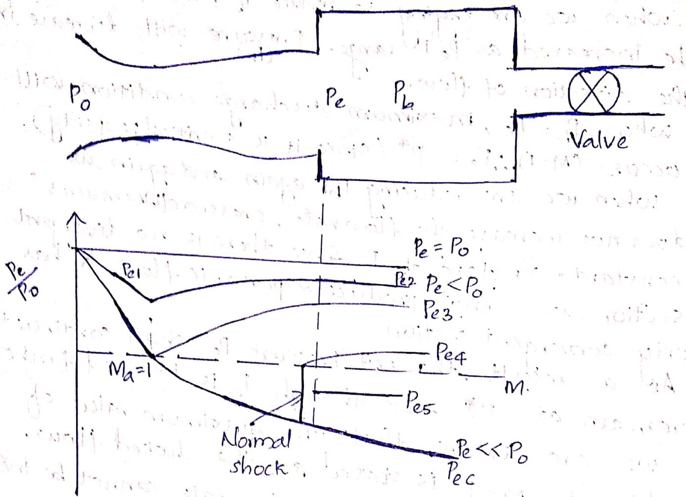
Nozzle is used to transfer pressure energy to kinetic energy. C-D Nozzle is used to produce supersonic flows.
