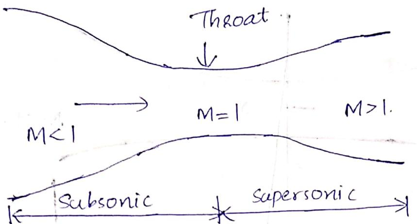
when throat diameter is optimized, we obtain maximum thrust. here gth is not considered.
